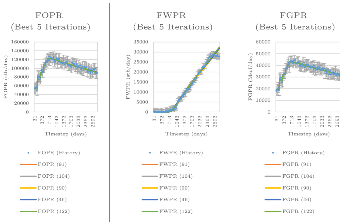
Figure 52 – Fluid flow response for FOPR (left), FWPR (middle) and FGPR (right) for GHM coupled with Adaptive Stochastic Sampling.
